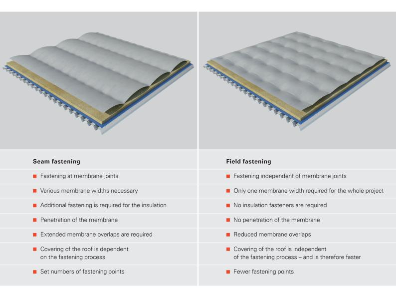
Whilst the field fastening technique application method for the attachment of single ply membrane is already used in the roofing industry; methods of attachment differ. The *isoweld™* field fastening system uses induction technology and offers a non-penetrating solution. Secure attachment is achieved through the welding of the membrane to a dedicated SFS intec stress plate.
